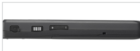
Earphone Jack, barcode scanner and volume
