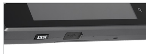
Trigger key and micro USB
