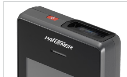
Power button barcode scanner window
